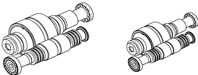
Figure 1. Illustration of Relative Sizes of API 613 Versus AGMA 6011 for Equivalent Design Conditions.
