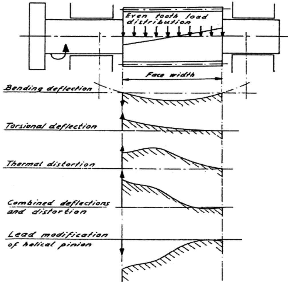
Figure H-1—Tooth Alignment (Lead) Modification of Helical Pinion
